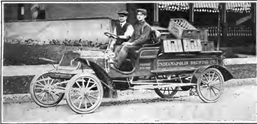
PREMIER OPEN EXPRESS WAGON WITH VERTICAL AIR-COOLED GASOLINE MOTOR.
